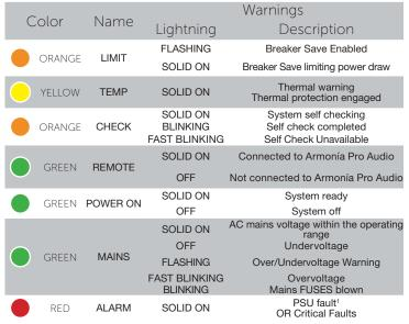
Red LED lights on in case of any kind of PSU fault that prevents normal operating.
