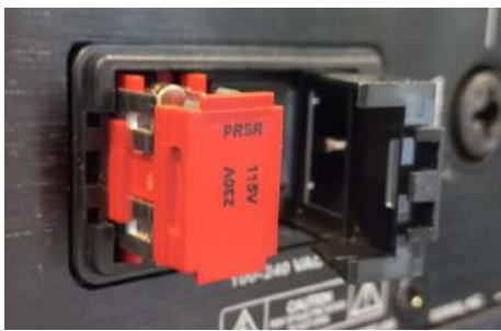
Step 3: Remove the fuse holder and rotate so that the voltage rating you require is oriented to the left.
