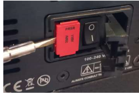
Step 2: Remove the fuse holder by using a flat head screwdriver as shown.
